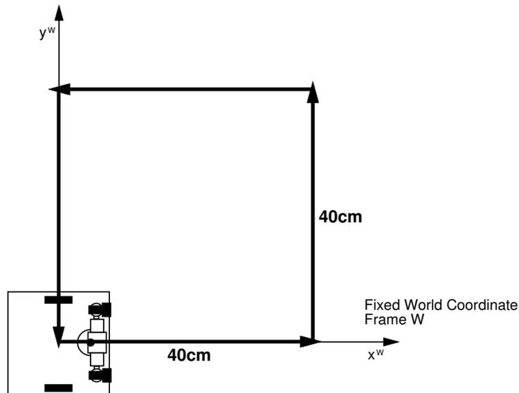
We have tape measures and scissors to borrow, and a big roll of stiff paper. Using a pen, **on your paper measure and mark out an accurate square course of side length 40cm for the robot to follow, starting at one corner, defining a coordinate frame as shown above.**
