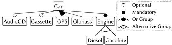
Figure 1: Feature model of the running example.
