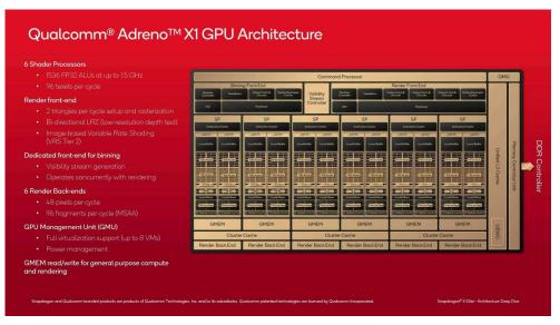
The Adreno X1 GPU is split up into 6 shader processor (SP) blocks, each offering 256 FP32 ALUs for a total of 1536 ALUs. With a peak clockspeed of 1.5GHz, this gives the integrated GPU on Snapdragon X a maximum throughput of 4.6 TFLOPS (with lesser amounts for lower-end SKUs).
