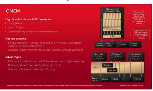
Key to making the binned rendering modes work is the GPU's GMEM, a 3MB SRAM block that serves as a very high bandwidth scratch pad for the GPU. Architecturally, GMEM is more than a cache, as it's decoupled from the system memory hierarchy, and the GPU can do virtually anything it wants with the memory (including using it as a cache, if need be).
