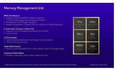
Conversely, Oryon's memory management unit is relatively straightforward. This is a fully-featured, modern MMU, and it supports even more esoteric features such as nested virtualization - which allows a guest virtual machine to host its own guest hypervisor for even more virtual machines farther down.
