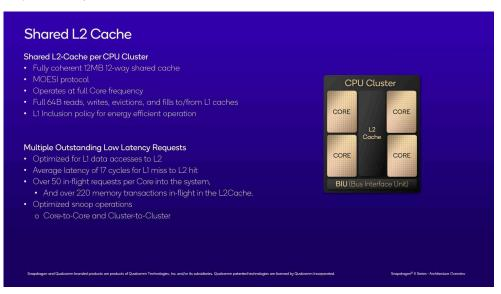
365 Unlike most CPU designs, Qualcomm is going with a slightly flatter cache hierarchy for Snapdragon X and the Oryon CPU core clusters. Rather than having a per-core L2 cache, the L2 cache is shared per 4 cores (this being very similar to how Intel shares the L2 cache on its E-core clusters). And this is a rather huge L2 cache, as well, at 12MB in size. The L2 cache is 12-way associative, and even with its large size, there's only a 17 cycle latency to access the L2 cache after an L1 miss.
