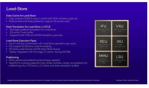
Branching off to its own slide, we have the data load/store units on Oryon. The core's load/store units are fully flexible, meaning that the 4 execution pipes can do any combination of loads and stores per cycle as needed. The load queues themselves can go up to 192 entries deep, while the store queues can go up to 26 entries. 517 And all fills are the full size of a cache line: 64 bytes.
