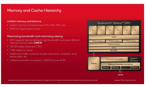
And when the Adreno X1 does need to go to system memory, it will go through its own remaining caches, before finally reaching the Snapdragon X's shared memory controller.
