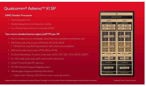
The individual shader processor blocks themselves are relatively customary, especially if you've seen an NVIDIA GPU architecture diagram. Each SP is further subdivided into two micro-pipes (micro shader pipe texture pipe, or uSPTP), which is helmed by its own dedicated scheduler and other resources such as local memory, load/store units, and texture units.
