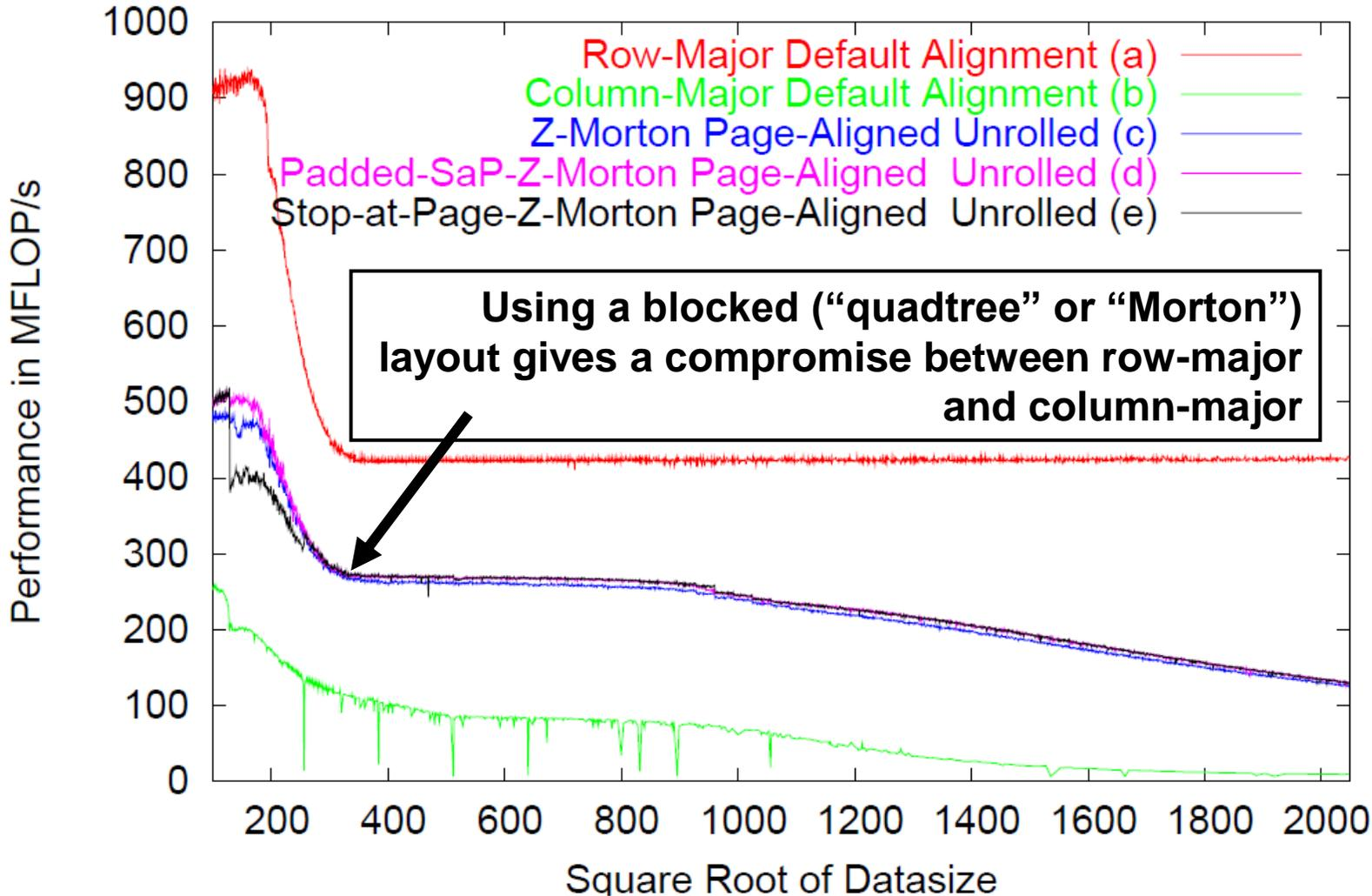
A variant of Morton-order layout is used for texture caching in some GPUs
