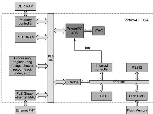
**Figure 5. System architecture.**
