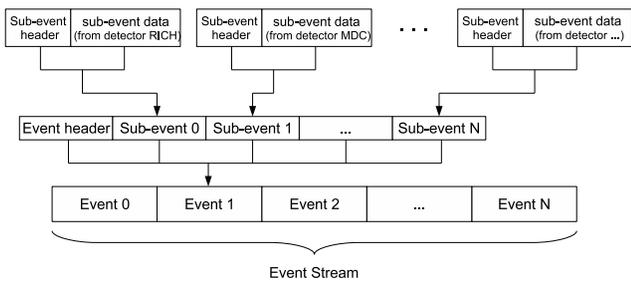
**Figure 4. Combining sub-events from various detectors into events.**
